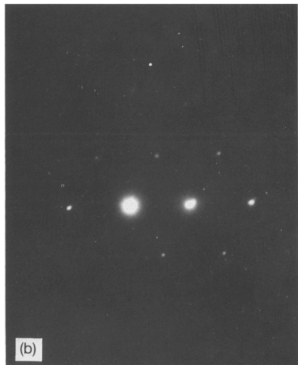
Figure 11 The electron diffraction patterns from the compound: (a) and (b) were obtained from the same phase at different angles.
